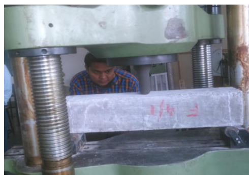
Fig.6 Flexural loading Test
